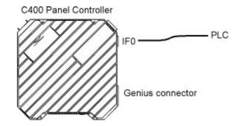
Figure 4 - 1. Panel to PLC Connections
